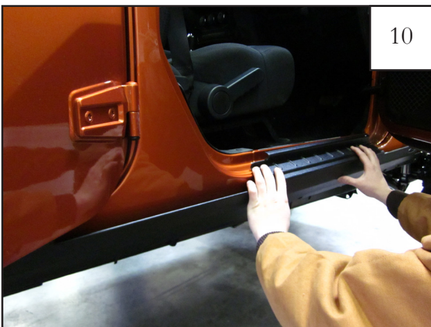
Press the part firmly into place following tape liner removal.
