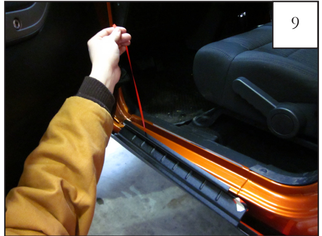
Remove all tape liners from the part in the order listed in step 1. As each liner is removed, press firmly on part at tape location to ensure adhesion.
