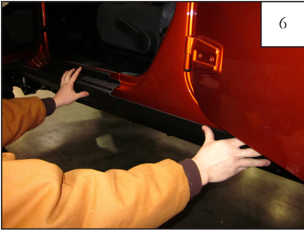
Place part on vehicle, making sure to line up edges of part with edges of vehicle and holes in part with clips installed in step 4. Ensure that all tape tabs are accessible.
