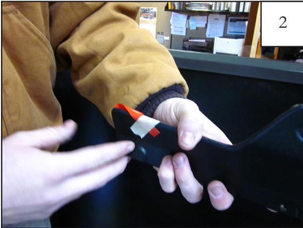
OPTIONAL: Using masking tape, secure tabs to the outside of part for easy access.
