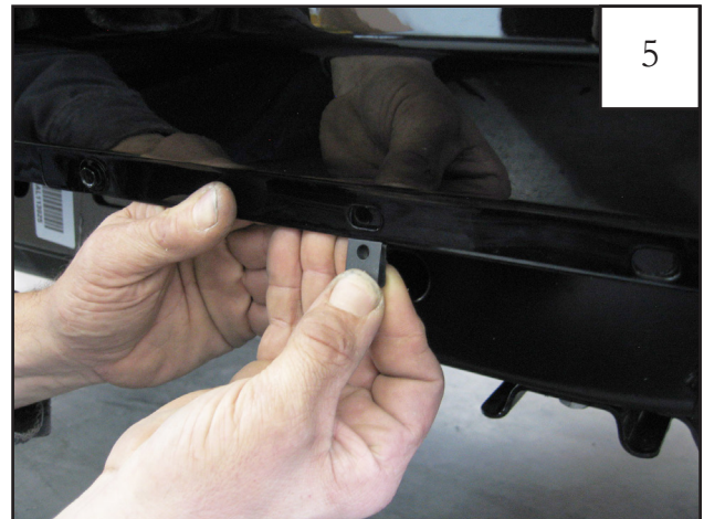
Place a clip over each hole with threaded portion of clip on the inside.
