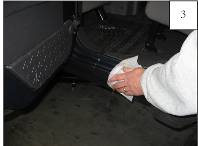
Open door, clean all dirt and debris from vehicle door sills, rocker panel, and beneath flares (if installed). Then, use supplied alcohol wipe (AD1-0008) where part will be positioned. NOTE: Temperature should be at least 60°F for proper tape adhesion.
